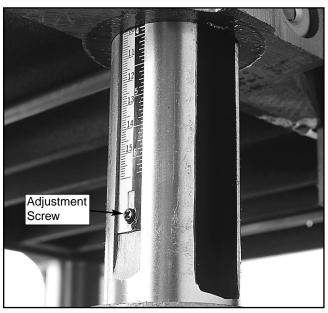
Figure 34. Thickness scale.
